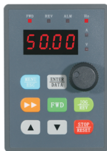
Figure C Running status, showing the operating status parameters
