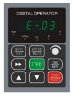
Fig. 4-5 Fault alarm display state
